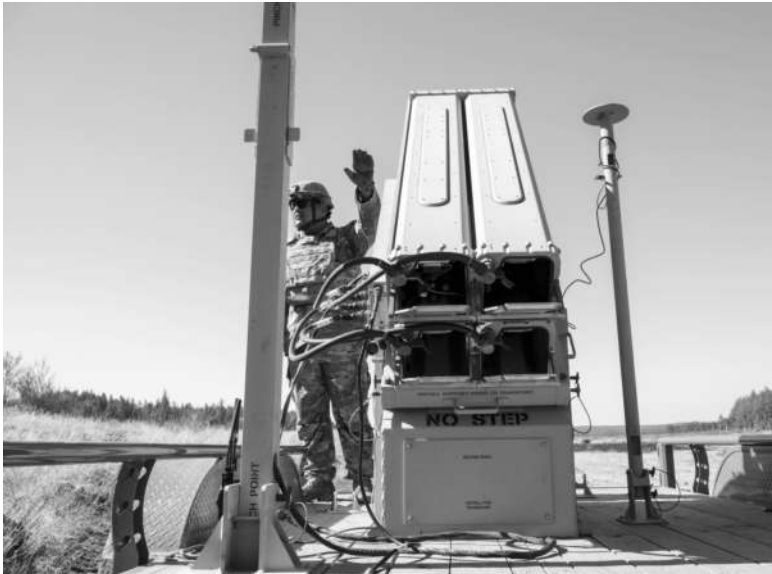
A battery of launch tubes for the Raytheon Coyote Block 3 Launch Effects drones are set up up at Joint Base Lewis-McChord.
